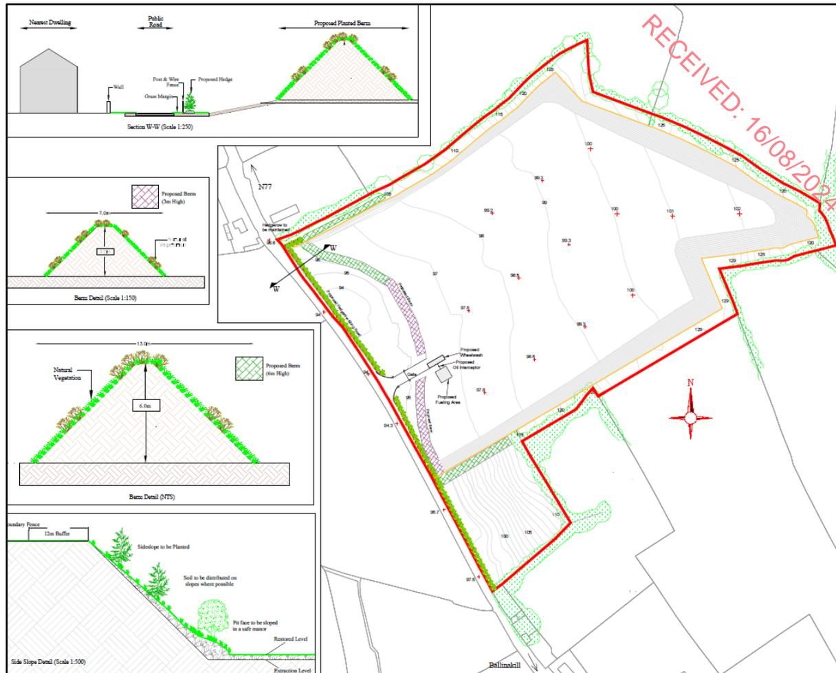
**Plate 10.3: Location and Section through Proposed Berms/ Barriers**
